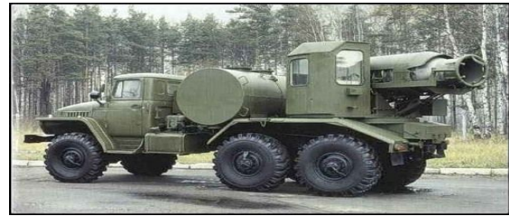
Figura 3 - TMS-65 Russian 6x6 Decontamination Vehicle
